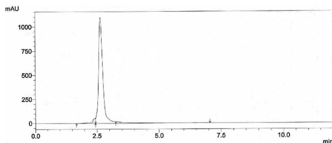
**Fig. 4.** HPLC chromatogram of GA conjugate with MetOMe (**IV**). Vydac C18 column (4.6 × 250 mm); mobile phase MeOH; flow rate, 1 mL/min; spectrophotometric diode-array detector at  $\lambda = 254$  nm. RT = 2.65 min; content of main compound  $96.2 \pm 0.5\%$ .
