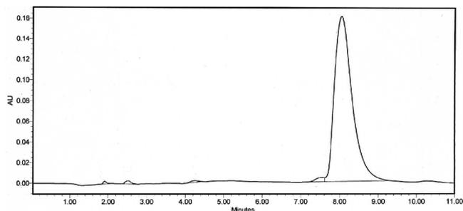
**Fig. 1.** HPLC chromatogram of glycyrrhizic acid (**I**). Atlantis C18 column (3.9 × 300 mm), mobile phase (MP) - MeOH-HOAc (0.3 N), 80:20 (vol%); MP flow rate, 1 mL/min; spectrophotometric diode-array detector at  $\lambda = 254$  nm. Retention time (RT), 8.04 min; content of main compound, 96.1 ± 0.5%.
