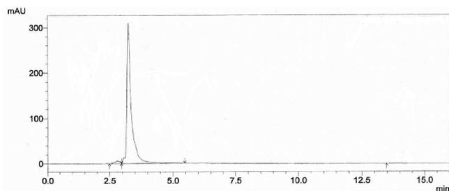
**Fig. 2.** HPLC chromatogram of trisodium salt of GA (**II**). Vydac C18 column (4.6 × 250 nm); mobile phase MeOH–HOAc (0.3 N), 80:20 (vol%); flow rate, 1 mL/min; spectrophotometric diode-array detector at  $\lambda = 254$  nm. RT = 3.23 min; content of main compound 97.5 ± 0.5%.
