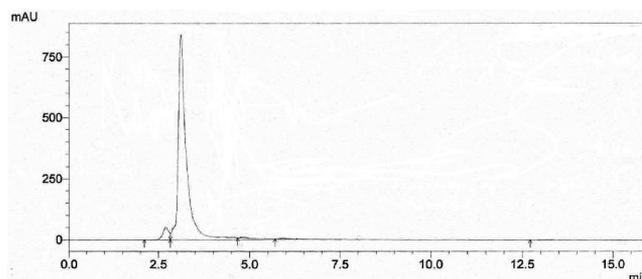
**Fig. 3.** HPLC chromatogram of sodium-dilithium salt of GA (**III**). Vydac C18 column (4.6 × 250 nm); mobile phase MeOH–HOAc (0.3 N), 80:20 (vol%); flow rate, 1 mL/min; spectrophotometric diode-array detector at  $\lambda = 254$  nm. RT = 3.11 min; content of main compound 94.7 ± 0.5%.
