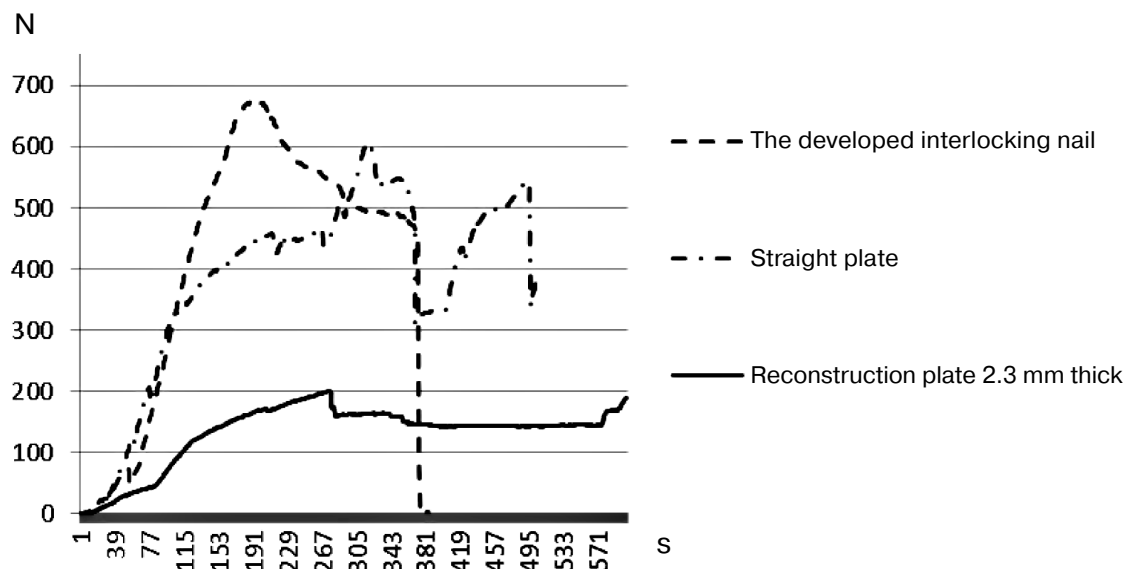
Fig. 3. Strength characteristics of the bone–implant–bone system in osteosynthesis of midshaft clavicular fractures under top-to-bottom loading in the frontal plane.
